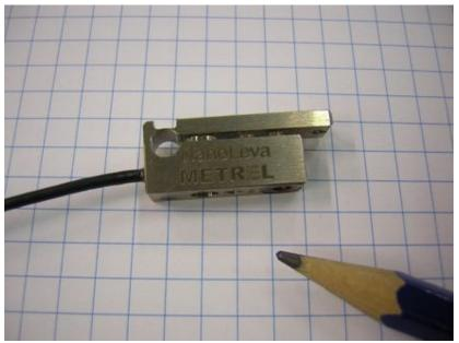
Figure No. 3- Small transducer called NanoLeva
