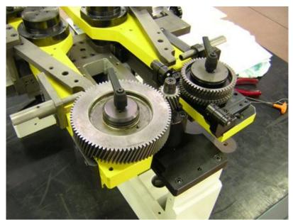
Figure No. 6b- Application of a carriage and special master for control of helix
