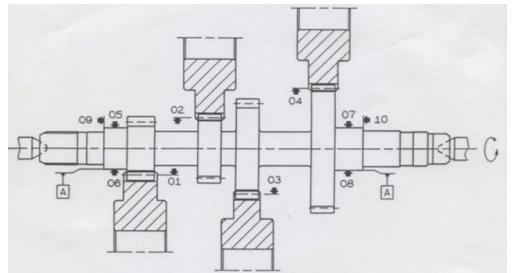
Fig.No.8- Measuring diagram of a shaft with 4 tooting.
