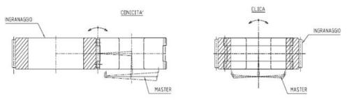
Figure No. 6a- Diagram of master floating movements for control of helix
