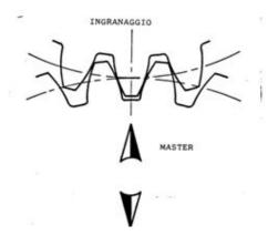
Figure No. 5- Operating principle of rolling gear tester at zero clearance
