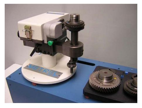
Fig. No. 1- Equipment for control of OBD dimension
