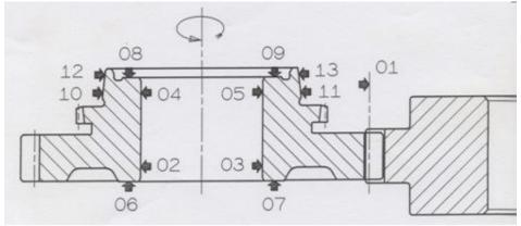
Fig.No.7- Measuring diagram of a gear with bore
